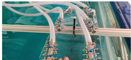
(B) 8 way manifolds to feed each of the 96 nozzles
